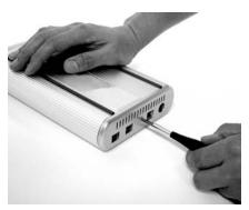
10. Secure the Back Panel with the 5mm diameter screw
